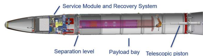
Figure 6: Sectional view of the Re-entry vehicle in a non-deployed configuration
